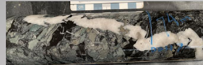
Quartz-ankerite-pyrite veinlet in heterolithic, black-matrix breccia from drill hole D1-21-7 at 74m. This single veinlet is responsible for an assay of 0.6 g/t Au over a 1 metre interval.
