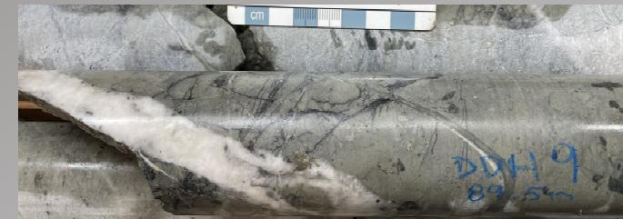
Quartz-ankerite-pyrite veinlet in highly altered sandstone from drill hole D1-21-9 at 89.5m. Three of these veinlets are responsible for an assay of 3.8 g/t Au over a 1 metre.
