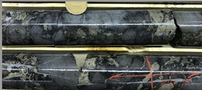
Heterolithic Black matrix breccia from drill hole D1-19-05 at 208.5 to 211.5m. Here, the breccia is clast supported with a great number of pyrite fragments.
