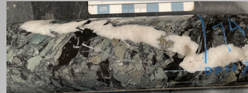
Quartz-ankerite-pyrite veinlet in heterolithic, black-matrix breccia from drill hole D1-21-7 at 74m. This single veinlet is responsible for an assay of 0.6 g/t Au over a 1 metre interval.
