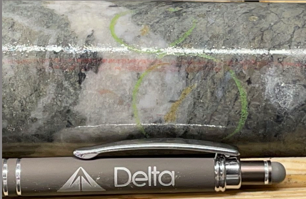
Quartz-Ankerite-pyrite-gold veinlet in the Feldspar-phyrlic intrusive from drill hole D2-22-18 at 314m.
