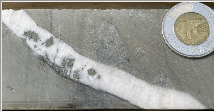
Quartz-ankerite-pyrite veinlet in sandstone from drill hole D1-21-10 at 79.9m. This single veinlet is responsible for an assay of 0.78 g/t Au over a 1 metre interval from 79m to 80m.
