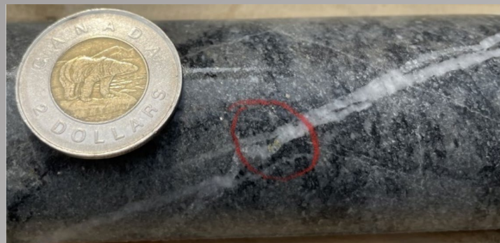
Quartz-ankerite-pyrite veinlet in sandstone from drill hole D1-21-10 at 102.3m with a speck of visible gold. This single veinlet is responsible for an assay of 2.9 g/t Au over a 1 metre interval from 79m to 80m.
